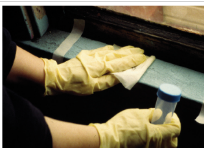
FIGURE 5.16 Dust testing a window sill to determine the presence of a friction hazard.
