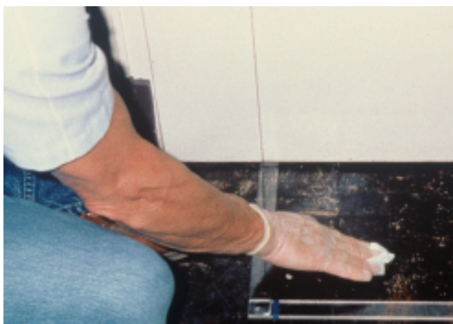
FIGURE 5.11e The second (vertical) pass.
