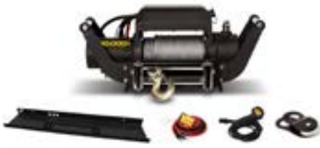
T37A. Champion 10,000 lbs. Winch Kit: Includes a Speed Mount 2" hitch adapter, 4-way roller fairlead, snatch block, 6' quick connect battery lead and a handheld remote. 53 points
