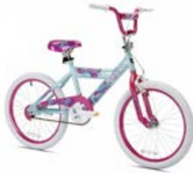
R21B. 20" Kent Lucky Star Girls Bike: Features a custom sturdy steel frame, a 4-bolt stem, front hand brake with rear coaster brake, steel rims and quick-release seat for easy adjustments. 13 points
